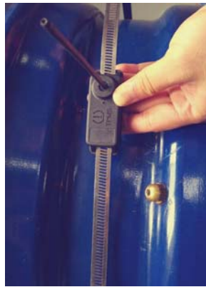
2、 Put the sensor on the steel tie
