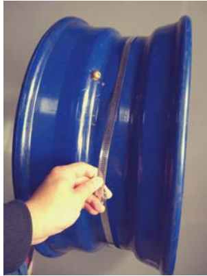
1、 The steel tie around the hub.
