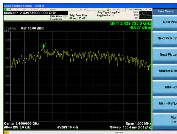
GFSK (BLE 1Mbps) MIDDLE CHANNEL
