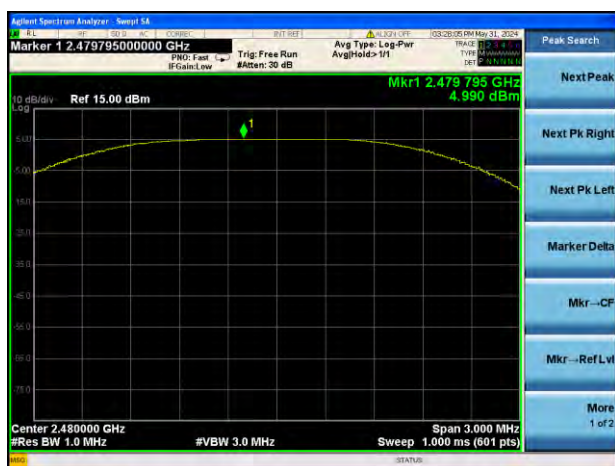
GFSK (BLE 1Mbps) HIGH CHANNEL
