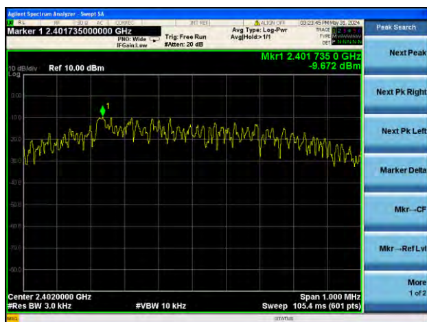
GFSK (BLE 1Mbps) LOW CHANNEL
