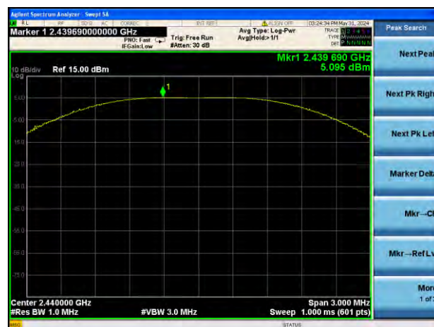
GFSK (BLE 1Mbps) MIDDLE CHANNEL
