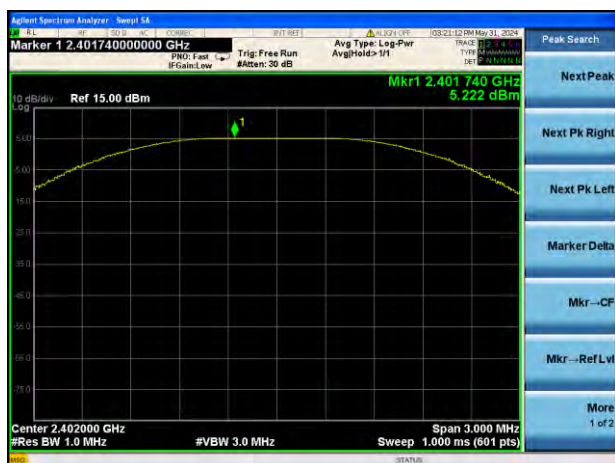
GFSK (BLE 1Mbps) LOW CHANNEL
