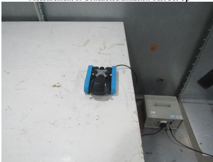
Measurement of Conducted Emission Test Set Up
