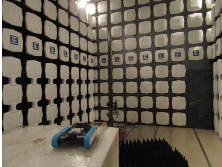
Measurement of Radiated Emission Test Set Up
