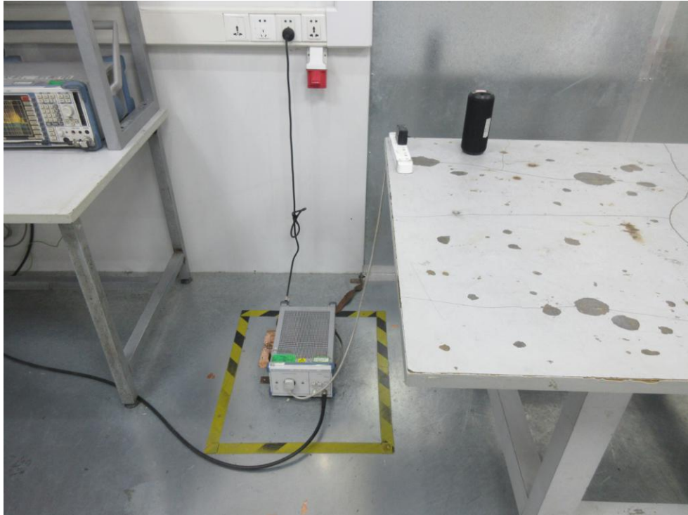
Photo of Conducted Emission Measurement
