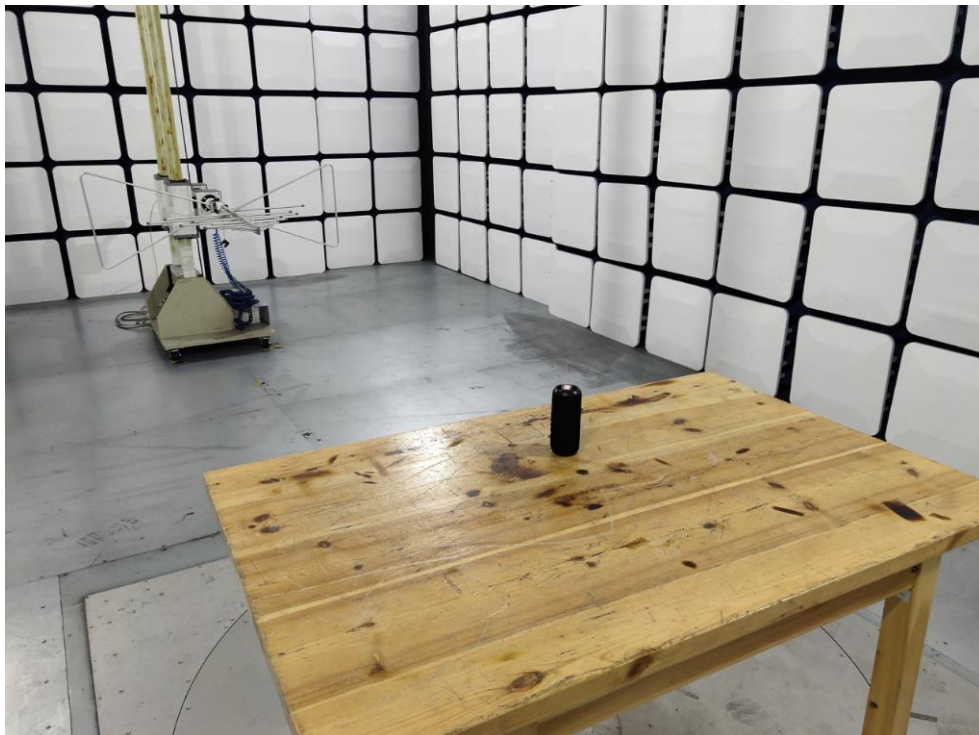
Photo of Radiation Emission Test
