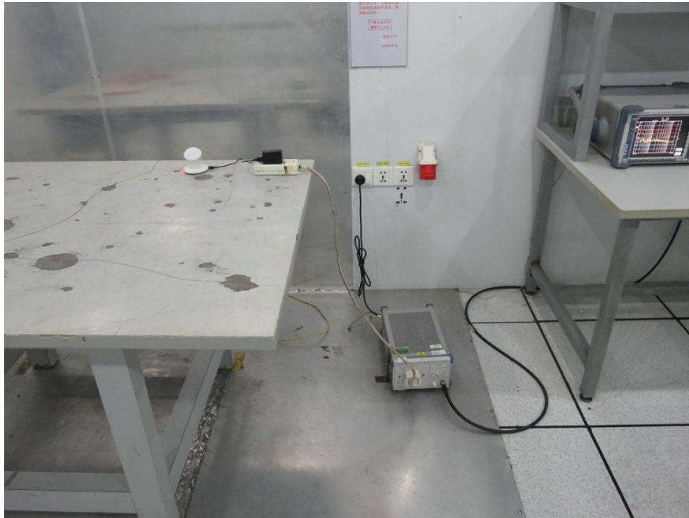
Photo of Conducted Emission Measurement
