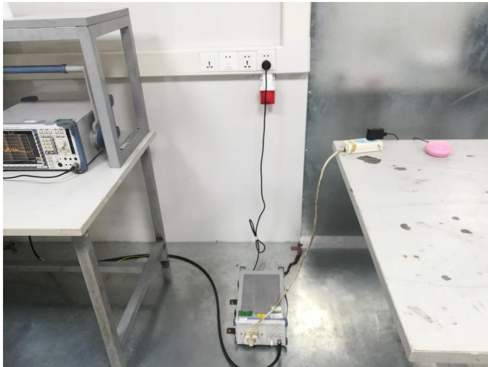
Photo of Conducted Emission Measurement
