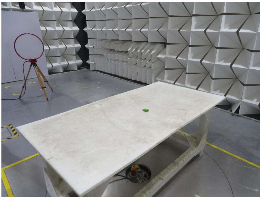
Radiated spurious emission Test Setup-1(9KHz-30MHz )
