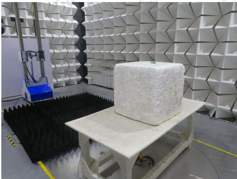
Radiated spurious emission Test Setup-3(Above 1GHz)
