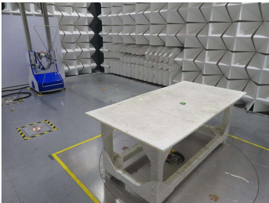
Radiated spurious emission Test Setup-2(30MHz-1GHz)
