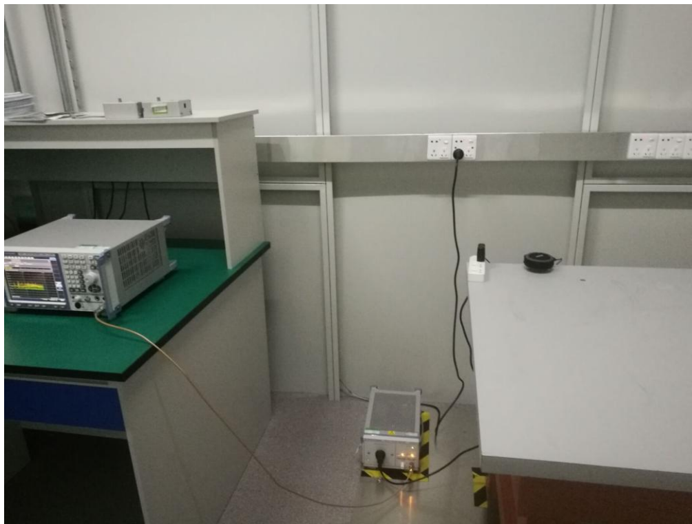
FCC RADIATED EMISSION TEST SETUP
