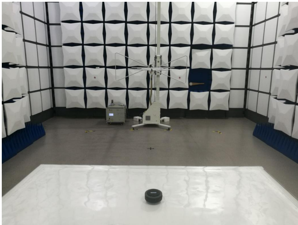
FCC RADIATED EMISSION TEST SETUP
