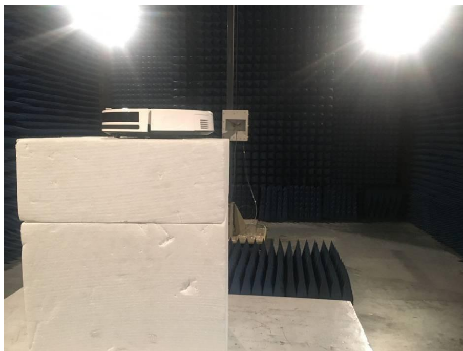
Above 1GHz: Test Height is 1.5m, the styrofoam block placed in the 0.8 m high test table
