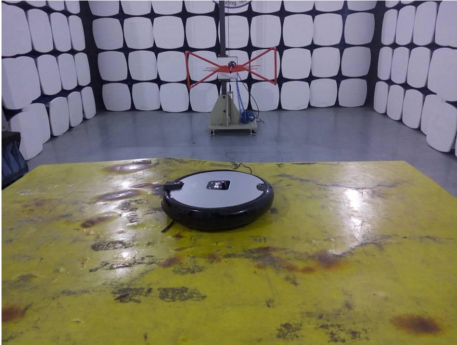
Below 1GHz: The EUT is placed in the 0.8 m high test table
