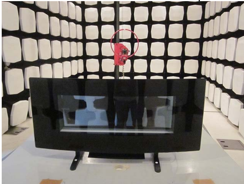
Measurement of Radiated Emission Test Set Up
