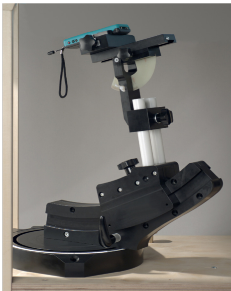
F-2. Device Holder for Transmitters
