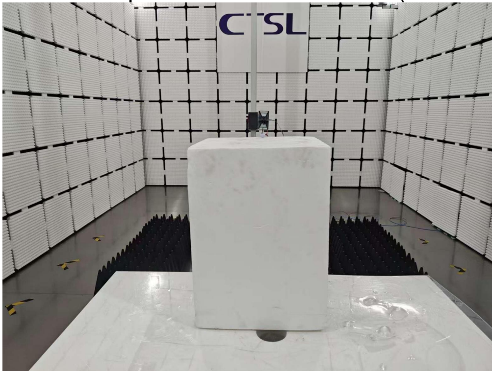
Photo 3 Test Setup Photos of Radiated Emission Test (Above 1GHz)
