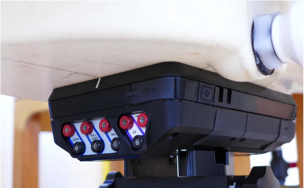
Fig. 9: Front of the device side towards the phantom, 0 mm distance.
