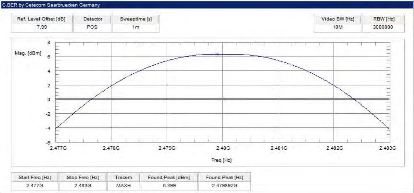
Plot 3: highest channel – 2480 MHz, GFSK modulation
