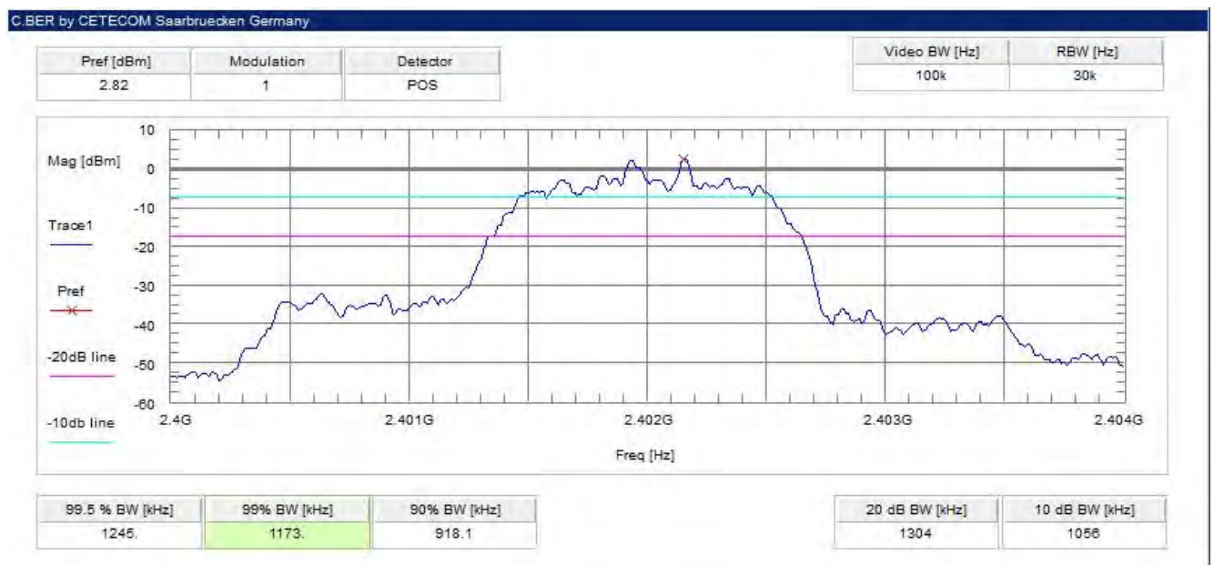
Plot 4: lowest channel – 2402 MHz, Pi / DQPSK modulation
