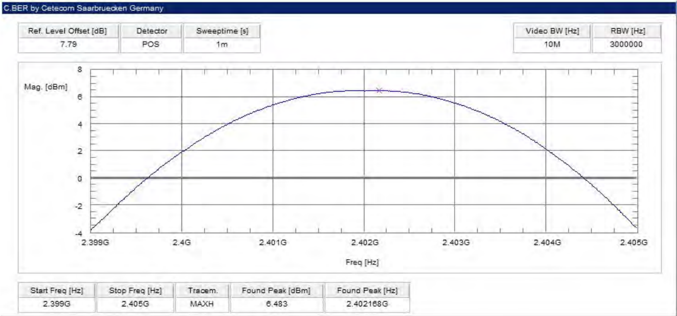
Plot 4: lowest channel – 2402 MHz, Pi / DQPSK modulation
