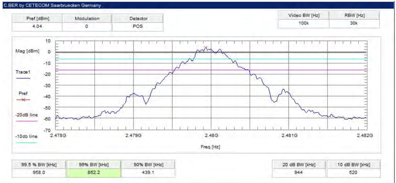
Plot 3: highest channel – 2480 MHz, GFSK modulation
