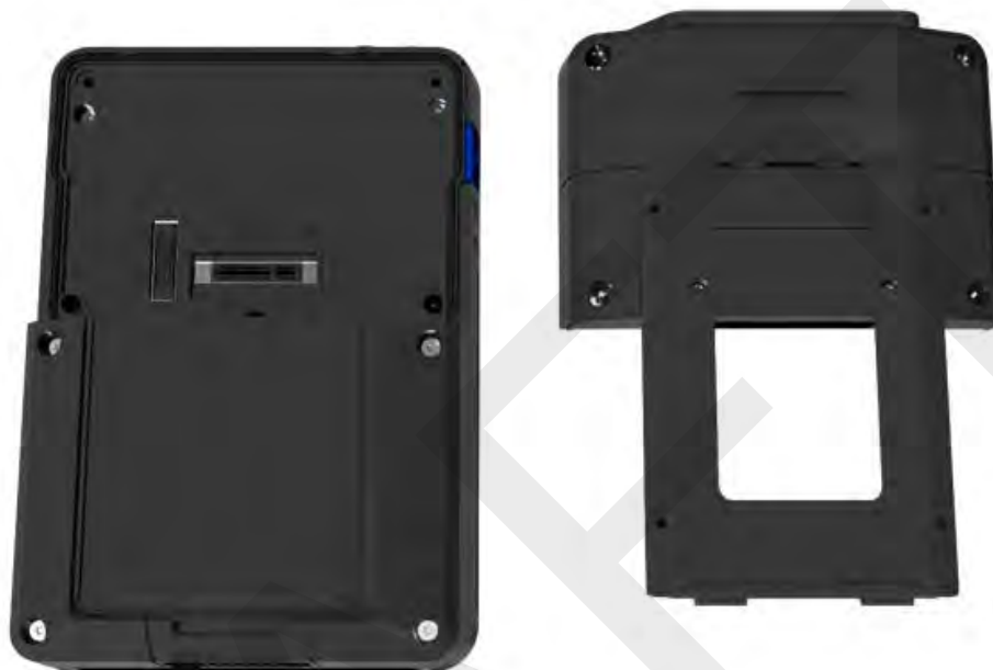
Figure 2-7: Trex unit with the communication module removed
