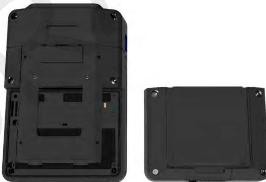
Figure 2-9: Trex unit with the power module removed
