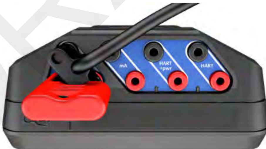
Figure 3-34: FOUNDATION fieldbus Power Plug attached to the Trex unit
