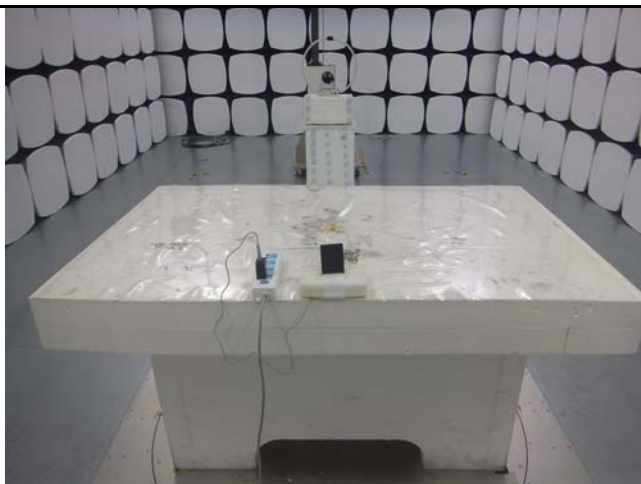
Radiated Spurious Emissions Test Setup 0.1MHz-30MHz
