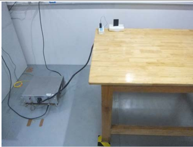
Conducted Emissions Test Setup – Front View
