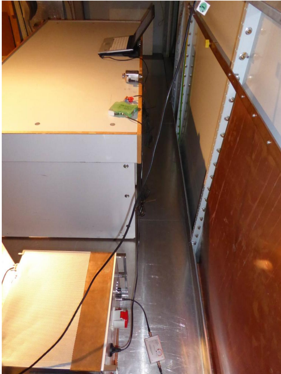
170014_42: Test setup – conducted emissions on power supply lines
