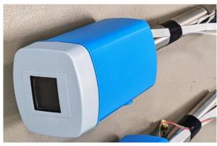
The EUT was supplied by 24 V DC during all tests. The EUT was set into water, the water/container was grounded, the data line was left open as declared by the applicant. During all test the EUT was operating in normal operation mode, Bluetooth was active and in idle mode (advertising/pairing mode).
