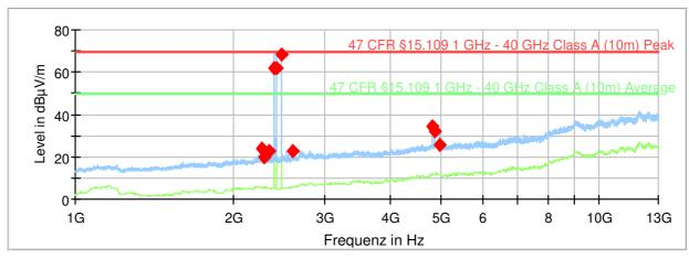
Preview Result 2-AVG Preview Result 1-PK+ 47 CFR §15.109 1 GHz - 40 GHz Class A (10m) Peak 47 CFR §15.109 1 GHz - 40 GHz Class A (10m) Average Final Result PK+ Final\_Result AVG
