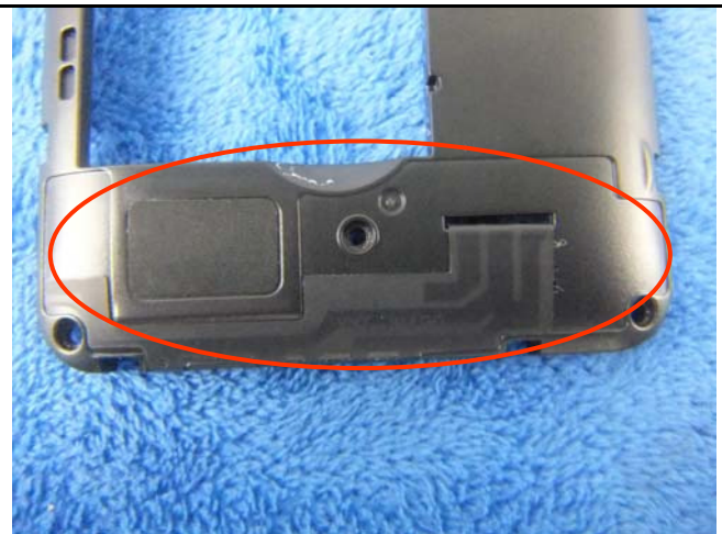
GSM/PCS/UMTS-FDD Antenna View
