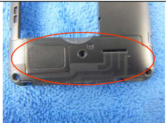
GSM/PCS/UMTS-FDD Antenna View
