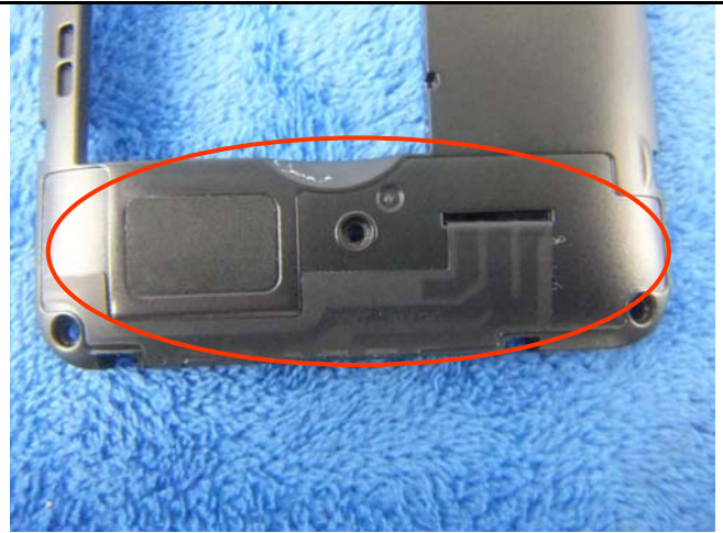
GSM/PCS/UMTS-FDD Antenna View
