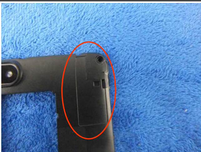
WIFI/BT/BLE/GPS - Antenna View
