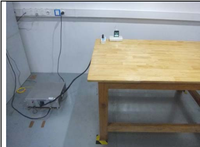
Conducted Emissions Test Setup Front View
