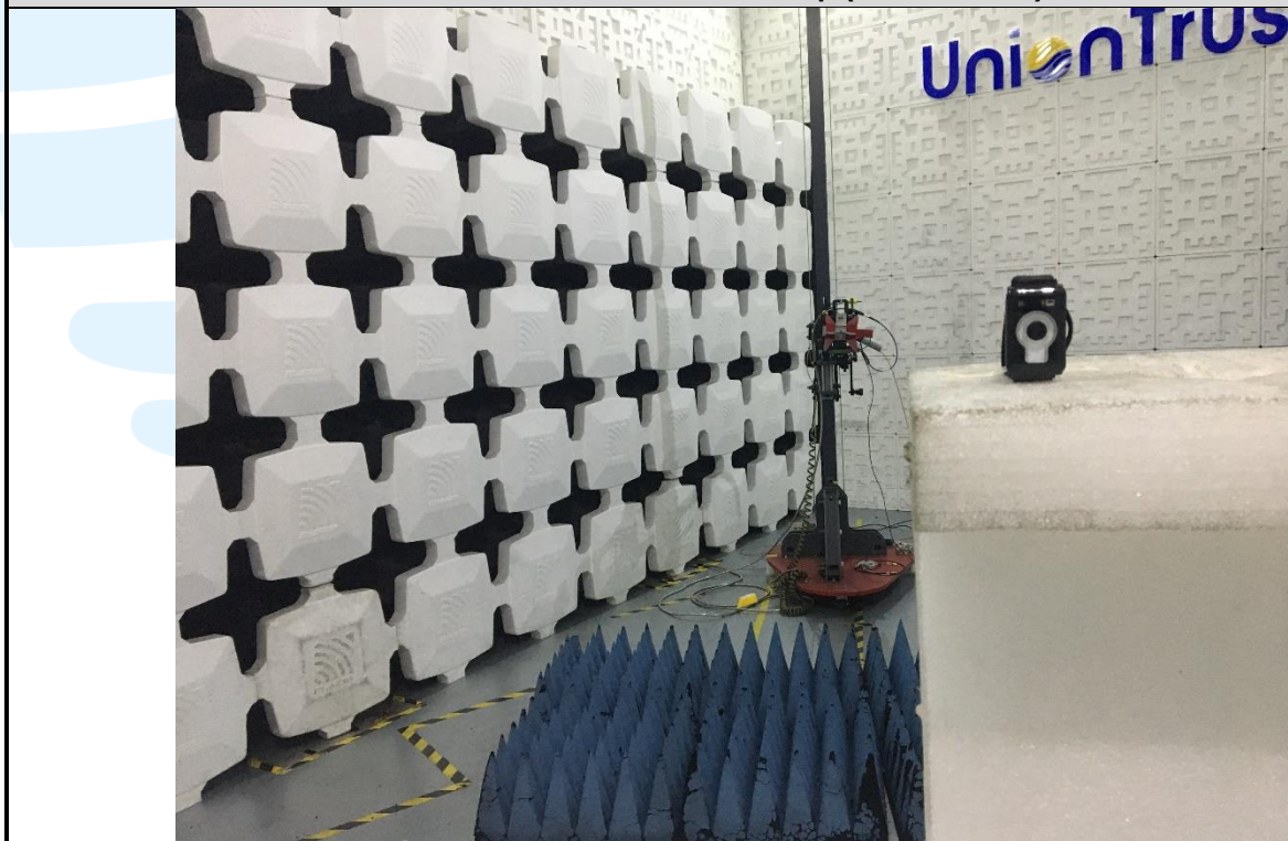
Radiated emission Test Setup (Above 1 GHz)
