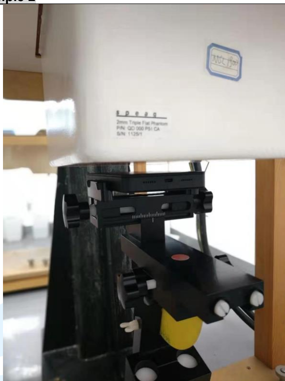
Rear Face of EUT with 1.0 cm Gap
