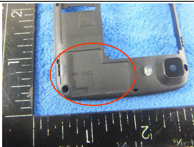
WIFI/BT/BLE/GPS - Antenna View
