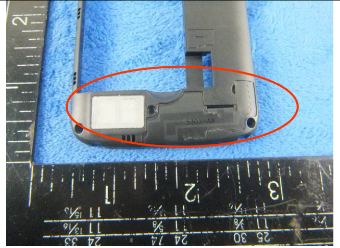
GSM/PCS/UMTS-FDD Antenna View
