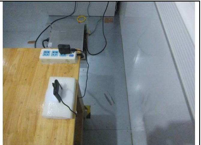
Conducted Emissions Test Setup Side View
