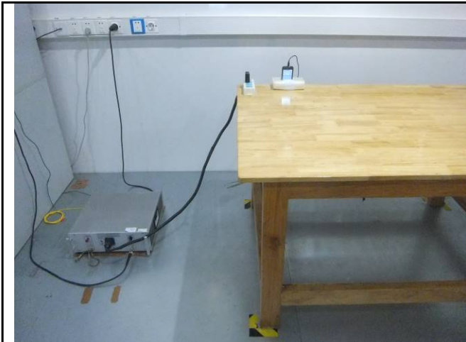
Conducted Emissions Test Setup Front View
