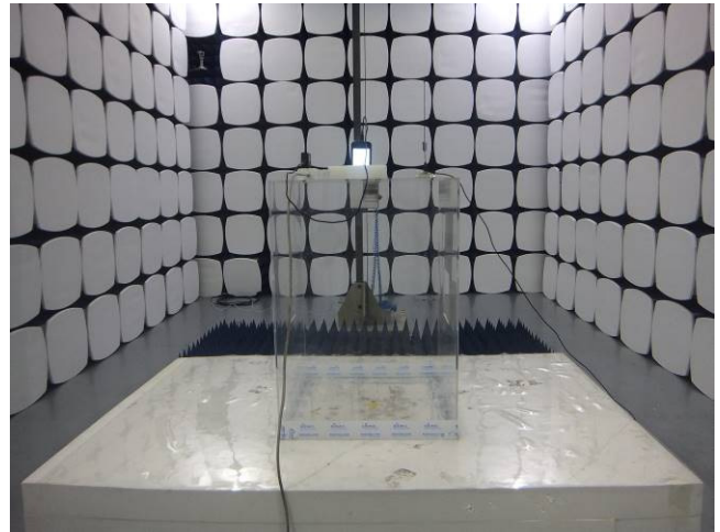
Radiated Spurious Emissions Test Setup Above 1GHz
