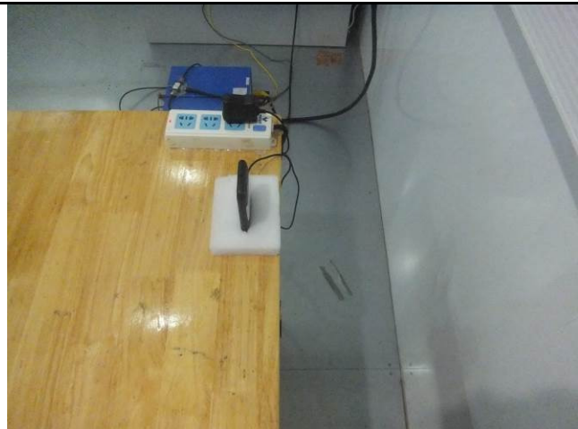
Conducted Emissions Test Setup Side View
