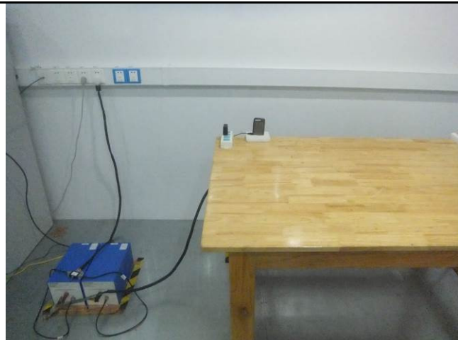
Conducted Emissions Test Setup Front View
