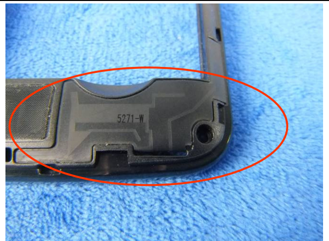
GSM/PCS/UMTS-FDD - Antenna View
