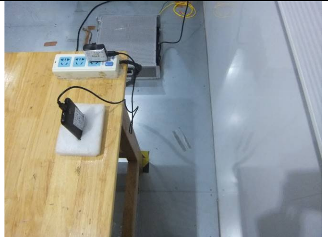
Conducted Emissions Test Setup Side View
