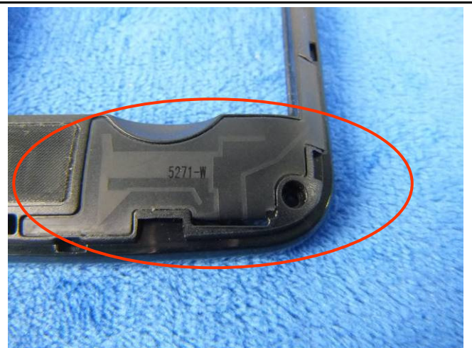
GSM/PCS/UMTS-FDD - Antenna View
