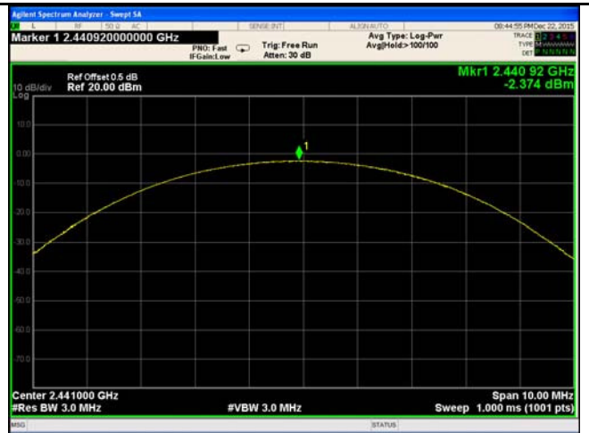
8DPSK Output power - Mid CH 2441
