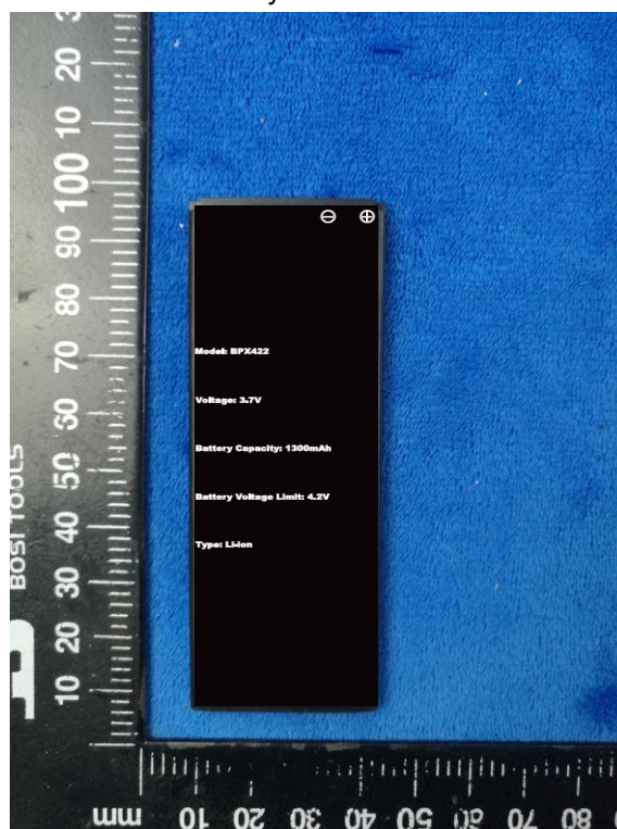
Battery - Front View
