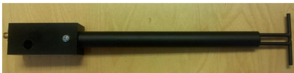
Figure 1 – MVG COMOSAR Validation Dipole
