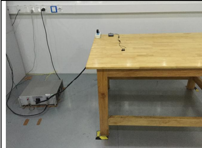
Conducted Emissions Test Setup Front View
