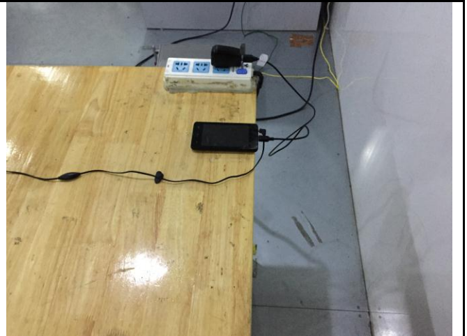
Conducted Emissions Test Setup Side View
