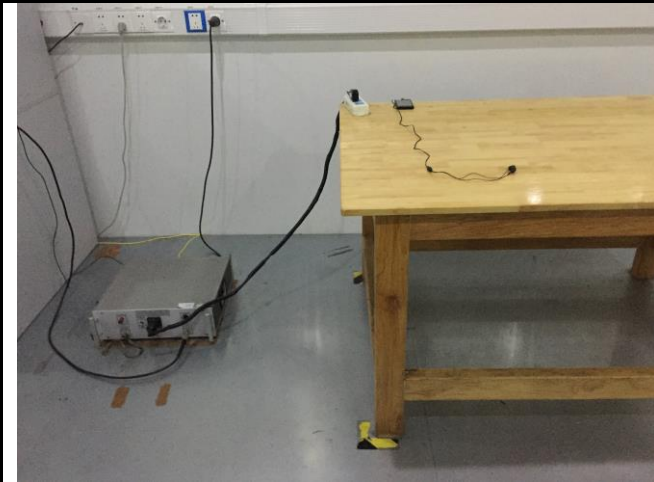
Conducted Emissions Test Setup Front View
