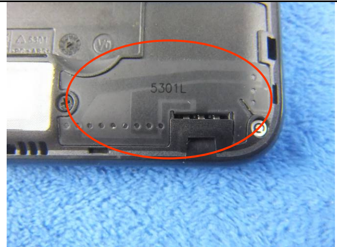
GSM/PCS/UMTS-FDD Antenna View
