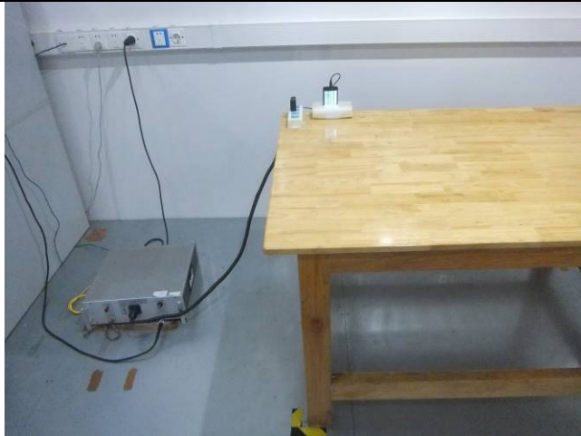
Conducted Emissions Test Setup Front View
