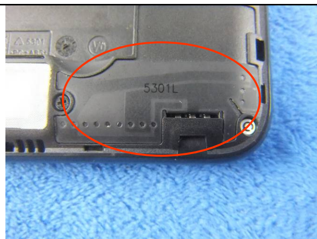
GSM/PCS/UMTS-FDD Antenna View
