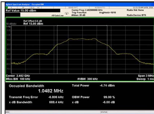
6dB Bandwidth - Low CH 2402
