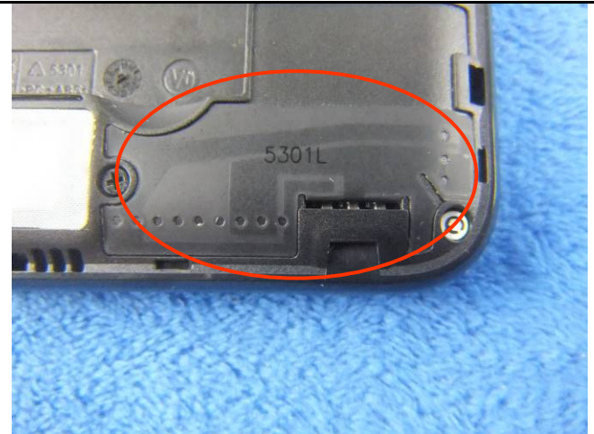
GSM/PCS/UMTS-FDD Antenna View
