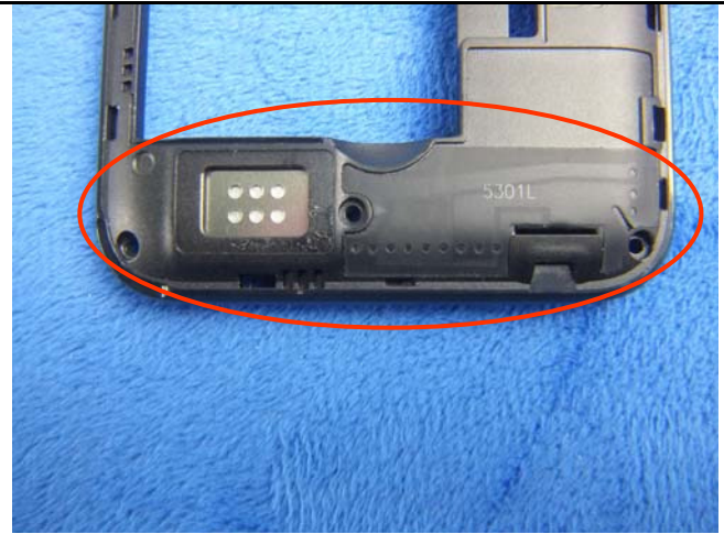
GSM/PCS/UMTS-FDD Antenna View
