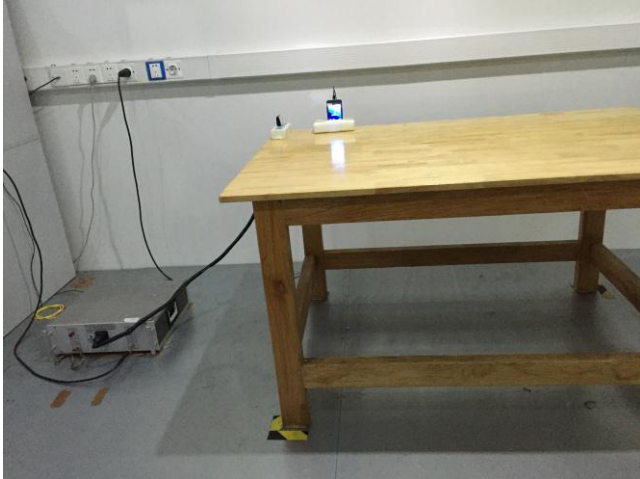
Conducted Emissions Test Setup Front View
