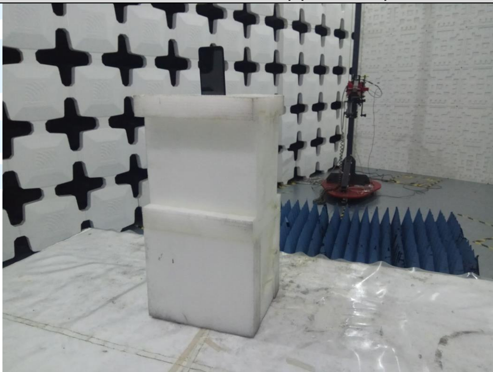
Radiated emission Test Setup (Above 1 GHz)
