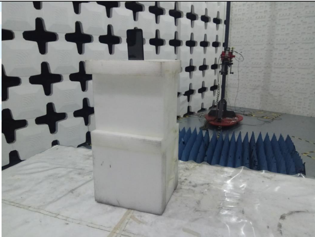
Radiated emission Test Setup (Above 1 GHz)
