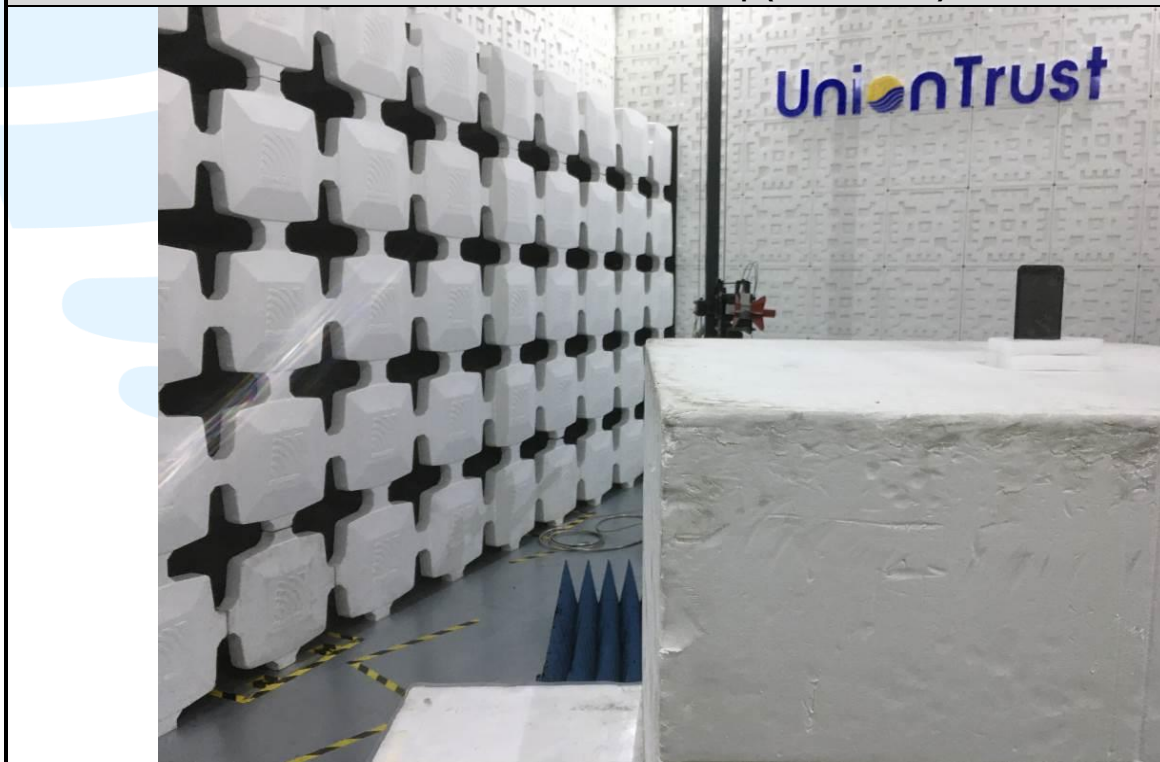
Radiated emission Test Setup (Above 1 GHz)
