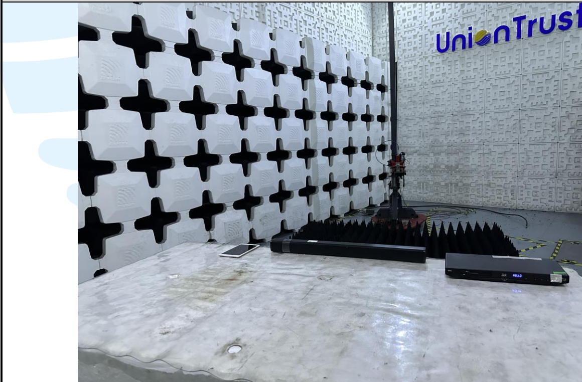
Radiated emission Test Setup-2 (Above 1 GHz)
