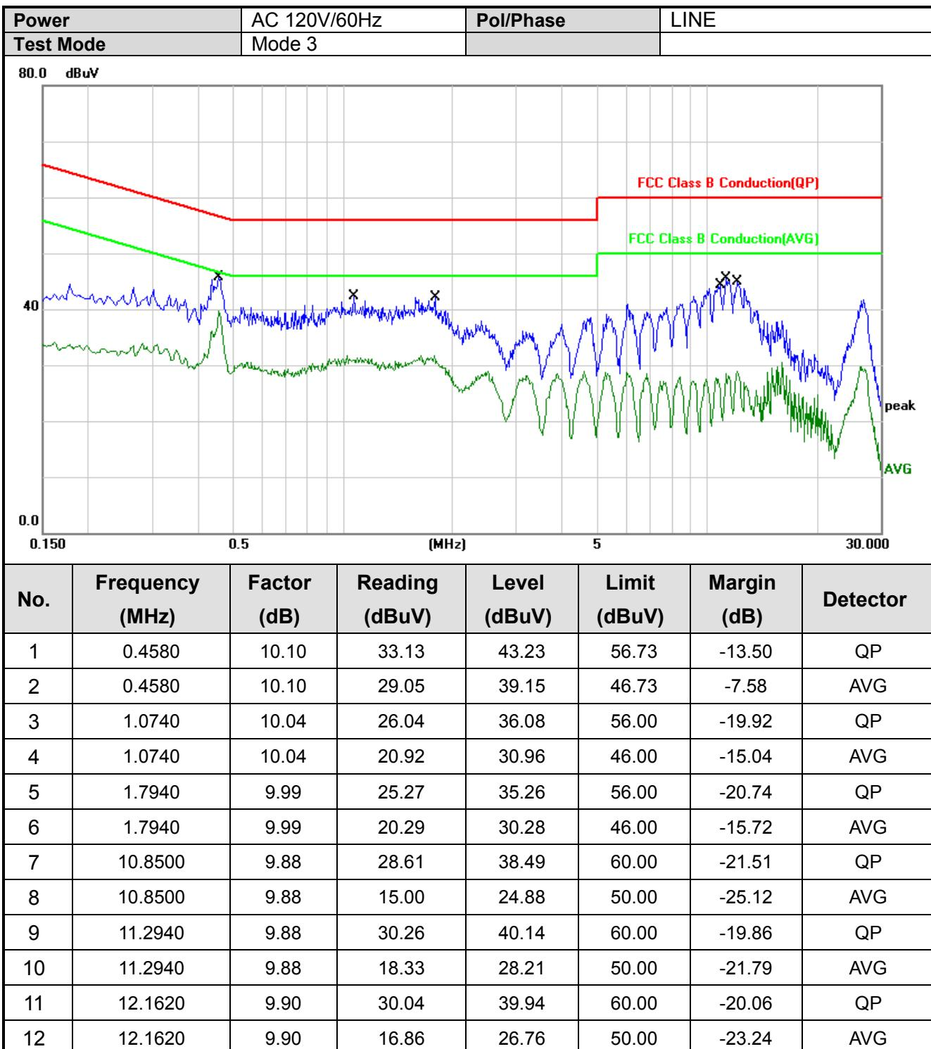
Note: Measurement Level = Reading Level + Correct Factor
