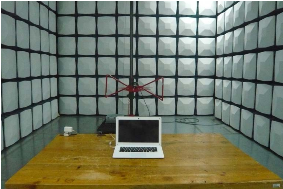
Radiated Emission View (Below 1GHz)
