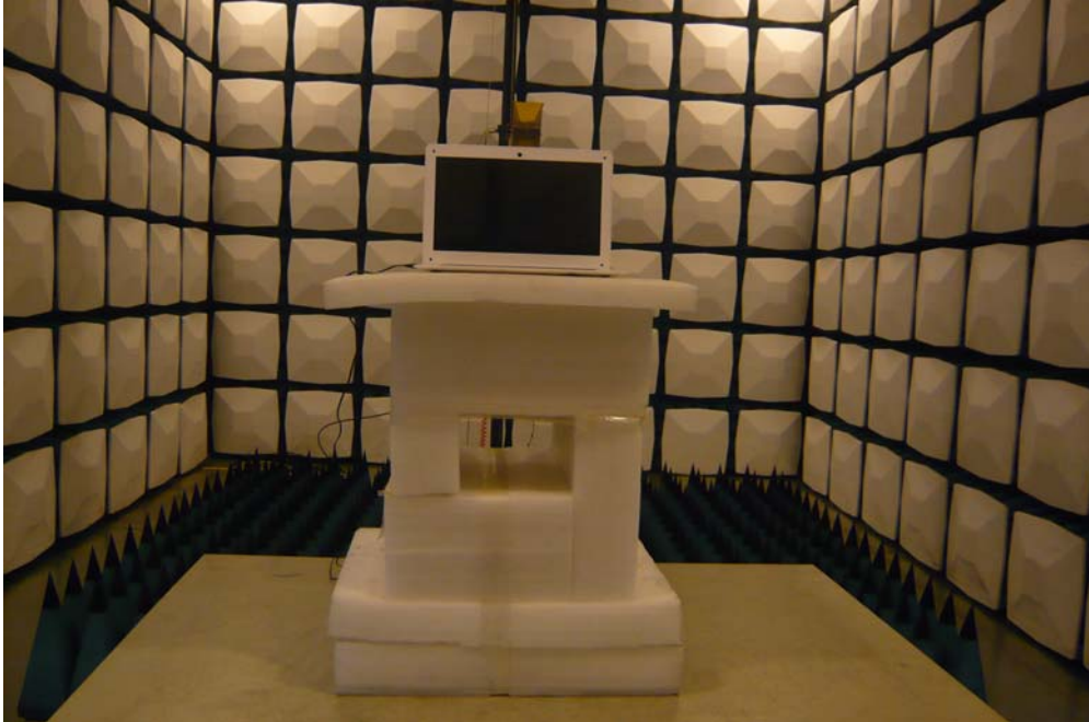
Radiated Emission View (Above 1GHz)
