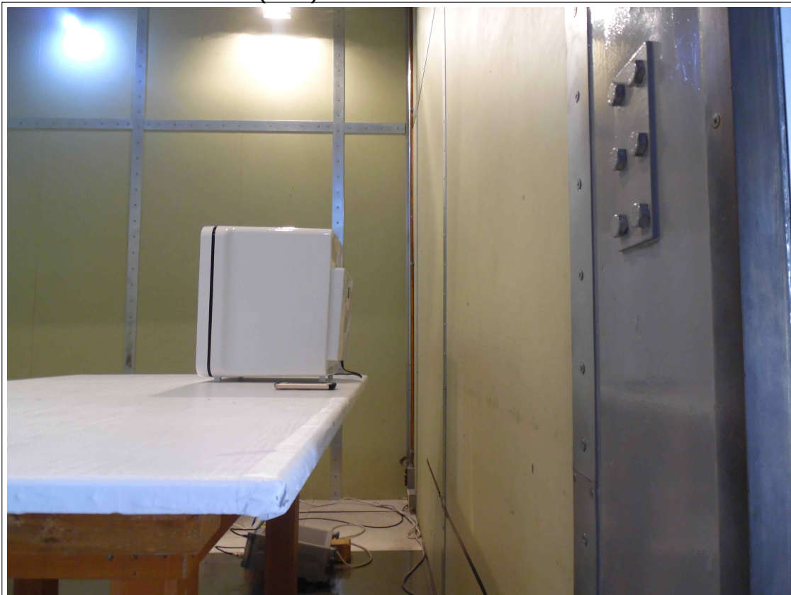
Conducted emission Test (Rear)
