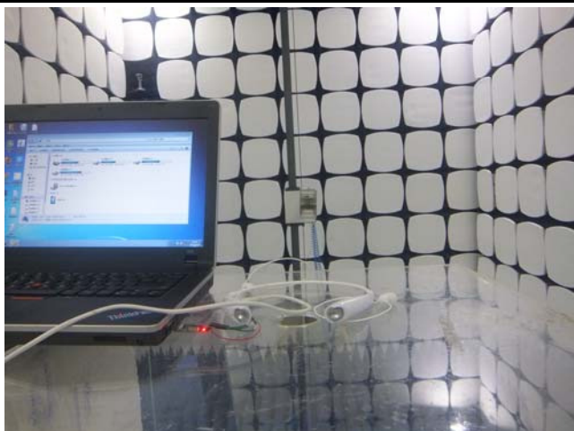
Radiated Spurious Emissions Test Above 1GHz
